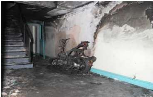
Clear burn pattern behind the scooter, Note rear tyre is still intact
